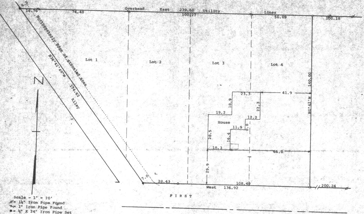
•= 4" X 24" Iron Pipe Set 0 = 1" X 24" Iron Pipe Set Bearings referenced to the north line of Pirst Street with the assumed bearing of West Survey ordered by: Realty World, Carmin Realtors
